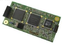
**Ethernet controller - ARL2300**: Allows remote control, 10MHz spectrum display, remote listening and audio recording of your AR6000 receiver, through the local network and Internet. Selectable audio bit rate.
